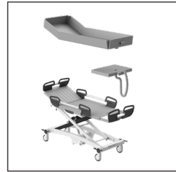
Figure 20 Disassembly of lying plate and mattress.
