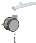
Figure 3 Tango XXL wheel exploded view
