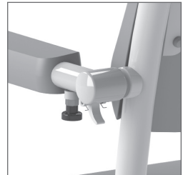
Figure 7. Armrest with dual locking.
